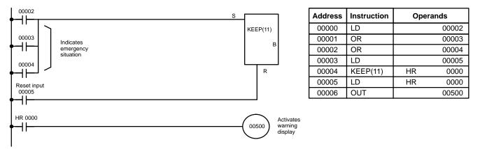
KEEP(11) can also be combined with TIM to produce delays in turning bits ON and OFF. Refer to *5-14-1 TIMER – TIM* for details.
